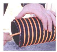
To strip the PVC, use wire cutters and partially cut the PVC to half depth. Fold the tip of PVC rod back and forth then pull on it to expose the static wire.
