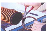
Use a knife to the hose to the desired length. Using a wire cutter cut the PVC helix away from the hose end.
