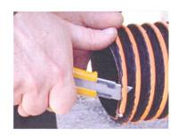
Using a carving knife, separate approximately 1-to 1-1/2" of rod from the carcass. Note: hold the knife with both ends to prevent injuries.
