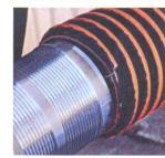
Once the wire is exposed, remove any excess wire. Bend the wire toward liner side and insert the stem.
