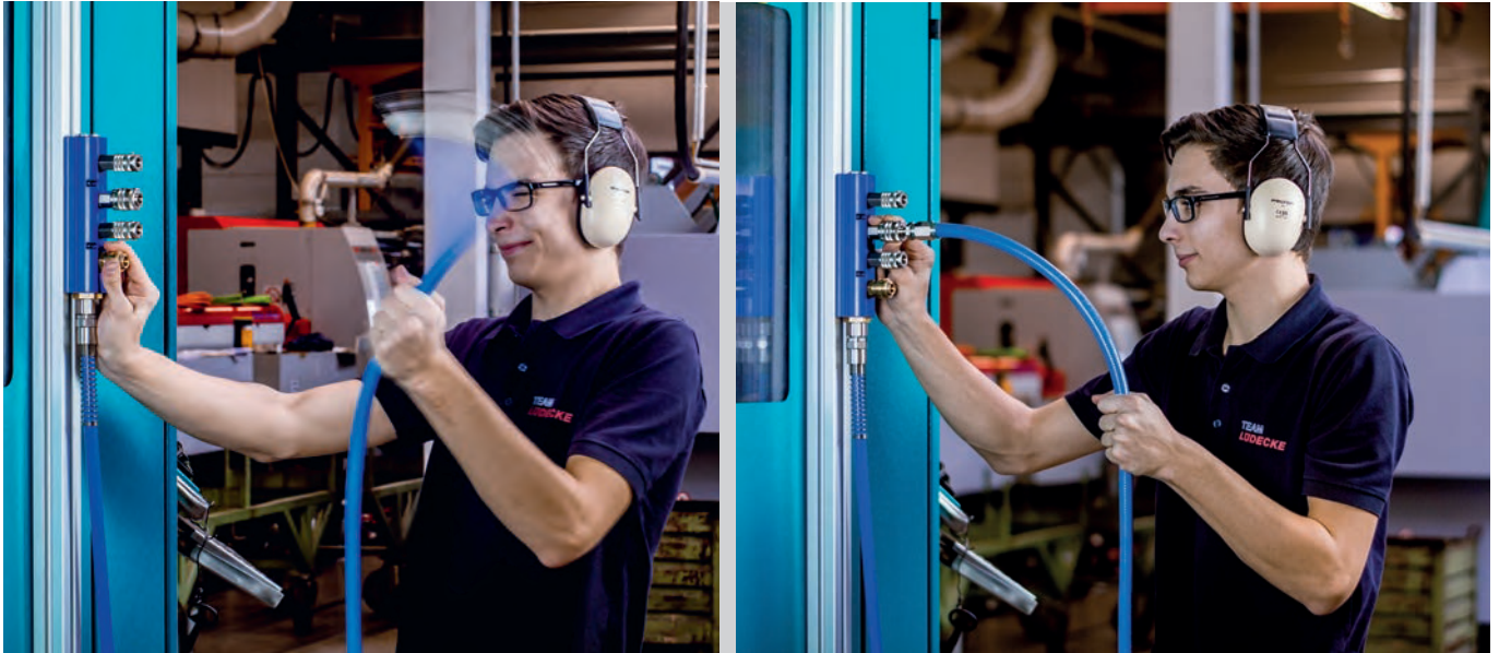
Whiplash-effect: high risk of injury when using compressed air - avoided through products from the LUDECKE SafeConnect-Line .
