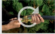
GEKA plus claw couplings are connected the same way as WaterProfi by **LUDECKE®** claw couplings. Push the two couplings together at 180° degrees opposite to each other until the seal faces touch. Afterwards, rotate one coupling half as far as it will go into the opposite direction of the other - the couplings lock into place.
