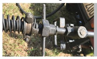
The **LUDECKE** hot tar screwings are made of steel/ malleable iron zincplated and yellow passivated (free of chrome VI) and are used to connect hoses to tar spraying equipment, lances, etc.
