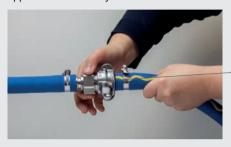
To ensure a perfect connection, the locking nut at the MODY-safety-screwing coupling is tightened manually.
