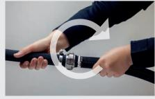
GEKA plus claw couplings are connected the same way as standard claw couplings. Push the two couplings together at 180° degrees opposite to each other until the seal faces touch. Afterwards, rotate one coupling half as far as it will go into the opposite direction of the other - the couplings lock into place.
