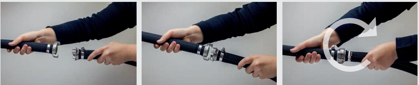
GEKA plus claw couplings are connected the same way as standard claw couplings. Push the two couplings together at 180° degrees opposite to each other until the seal faces touch. Afterwards, rotate one coupling half as far as it will go into the opposite direction of the other - the couplings lock into place.
