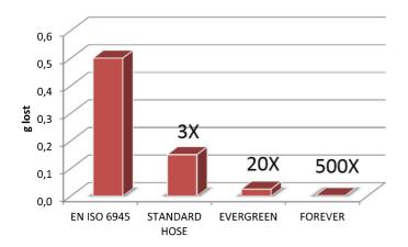
When tested in accordance with ISO 6945 specification, EVERGREEN rubber cover shows abrasion resistance up to 20 times better results
